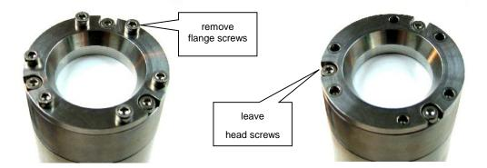
remove the flange by prying it open carefully. At the beginning it might be hard to pull, after a few mm, once the first seal-ring appear, it pulls out easily. Avoid slanting.
