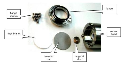
The flange has a side seal-ring and a membrane seal-ring.
