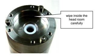
Put back in place first the support ring, then the sintered disc, and finally a new membrane. Place the membrane as flat as possible (smooth with finger is possible)
